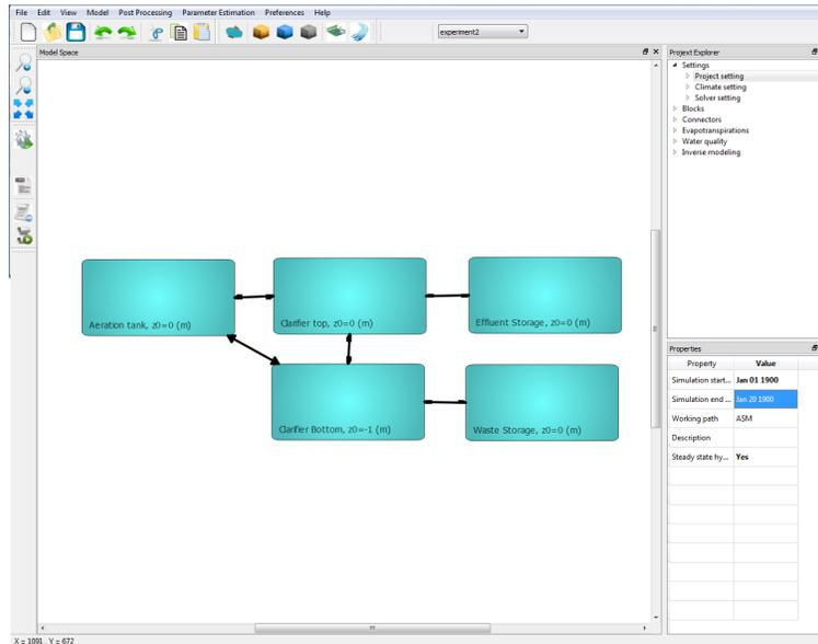
Figure 2: Activated sludge model configuration in GIFMod
